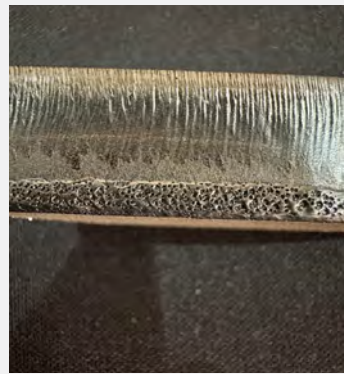
HARDOX 12 mm metal cut with LASER using Oxygen. In this photo we can clearly see the burning of metal piece at the bottom portion of the work piece.
