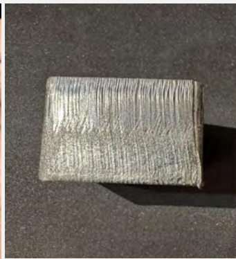
30mm thick A36 metal cut with LASER using Oxygen.
