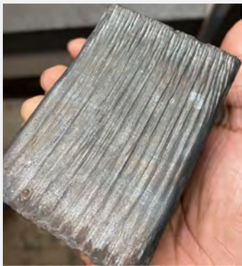
80mm thick A36 metal cut with LASER using Oxygen.
