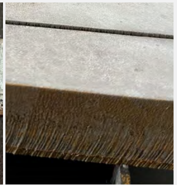
HARDOX 450 - 40mm HARDOZ material cut with waterjet machine. This photo clearly shows that no burns occur during the cutting process.
