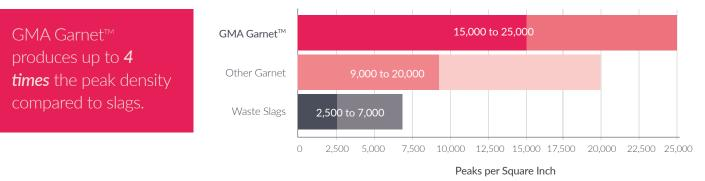
Source: Comparative Study of Prevalent Blasting Abrasives in the US Market, April 2019. Average Results from typical 80 Mesh and 30/60 Mesh abrasives on carbon steel which had light mill scale and surface rust.
