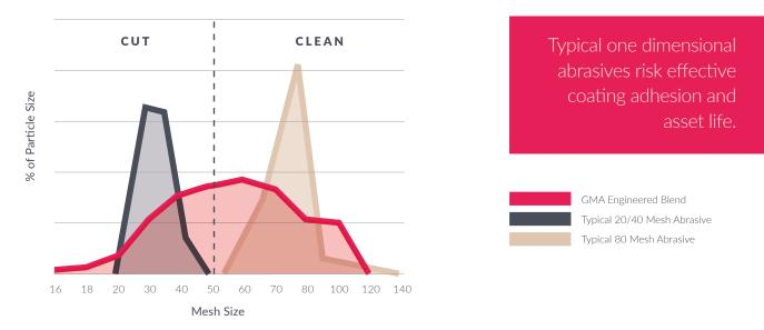
A wider particle size distribution enables effective coating removal and profile depth by coarse particles, enhanced by the efficiency and cleaning benefits of the finer particles.
