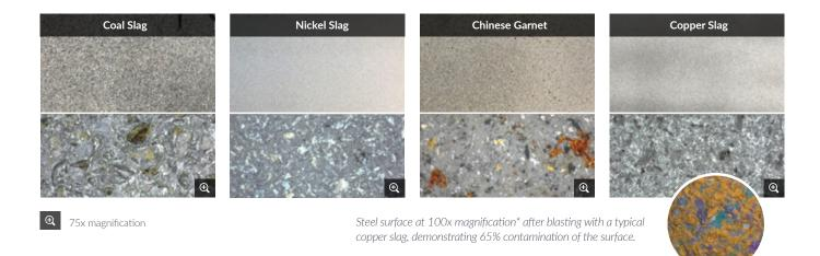
Measured using Scanning Electron Microscope (SEM), Backscattered Electron (BSE) and digital analysis.
