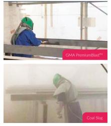
\*Production and consumption rates may vary based on nozzle size, pressure at the nozzle, standoff distance, abrasive metering, equipment quality, surface type, coating type and thickness. The blasting rates are achieved by setting the nozzle pressure to operate within the range of 95 psi – 100 psi. GMA will work with you to produce optimum performance on blasting jobs, reducing time and cost, and producing the best surface result for any coating.
